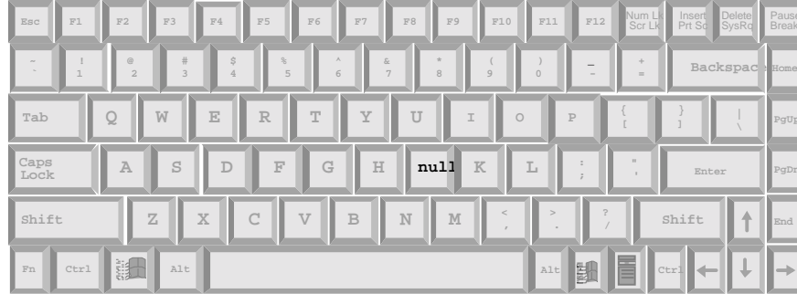
Example 3: When the Fn layout is active, the key acts as a "null" key.
