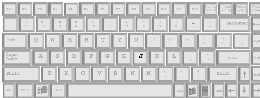
Example 1: “Alternate layouts” key number DBh acts as the “J” when the QWERTY layout is active.
